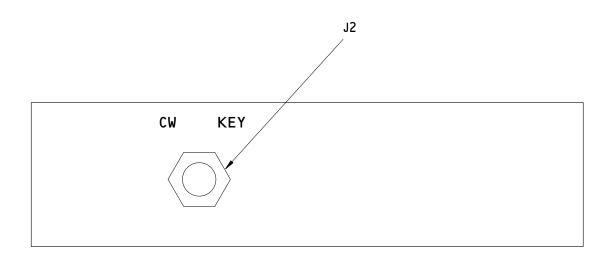
233T4252-1 HF Comm - CW Jack Panel Assembly Component Location Figure 1
